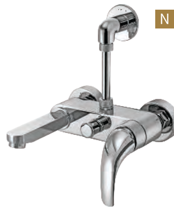
QDS-3102 LB Side operated single lever wall mixer with 'I' shaped tubular bend set for overhead shower
